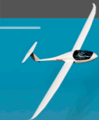
Taurus Electro world's first two seat electric aircraft
