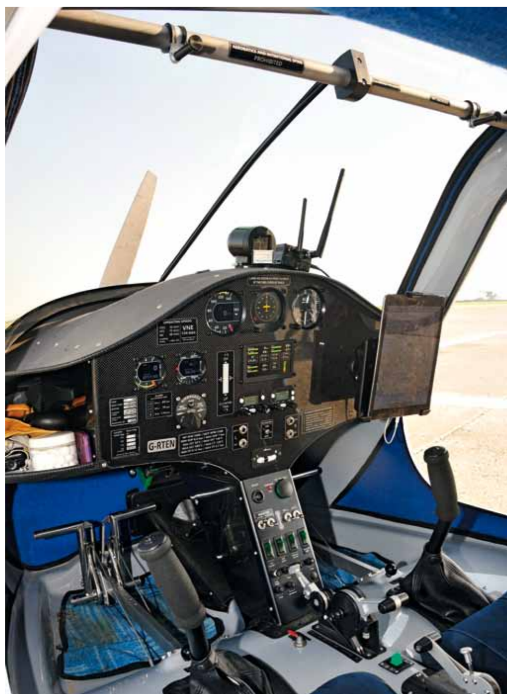
ABOVE: well-positioned digital-analogue flight instruments top the very 21st century panel. Design and quality of the choke, throttle and brake quadrants is superb
