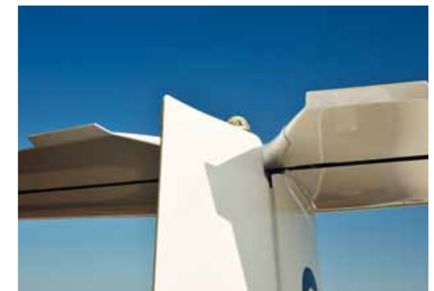
The elevator is cambered to produce a downforce on the tailplane and the fixed tabs are there to trim out control loading
