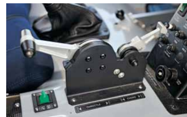
TOP TO BOTTOM: the 'handbrake' lever operates the flaperons, airbrakes being extended at '+2' when set to 'auto'; combined brake/parking brake hand lever; and (from left in photo) electric trim switch and the beautifully engineered throttle and choke levers
