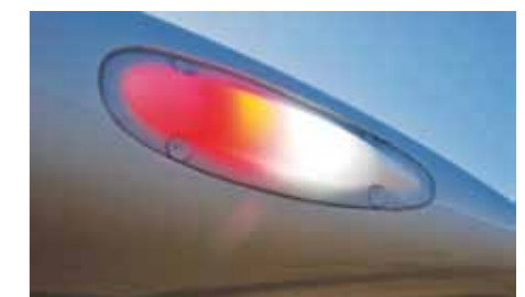
Neat detail unusual for a microlight: combined wing-tip navigation and landing lights
