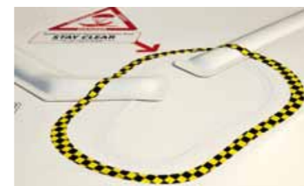
Near 'zero-zero' capability: the BRS 'chute deployment minima are 200ft agl and 25kt
