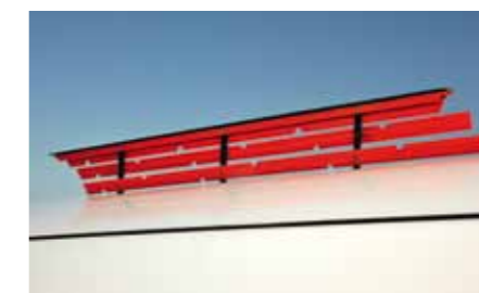
Airbrakes are designed to pop out automatically when the flaperons are fully drooped
